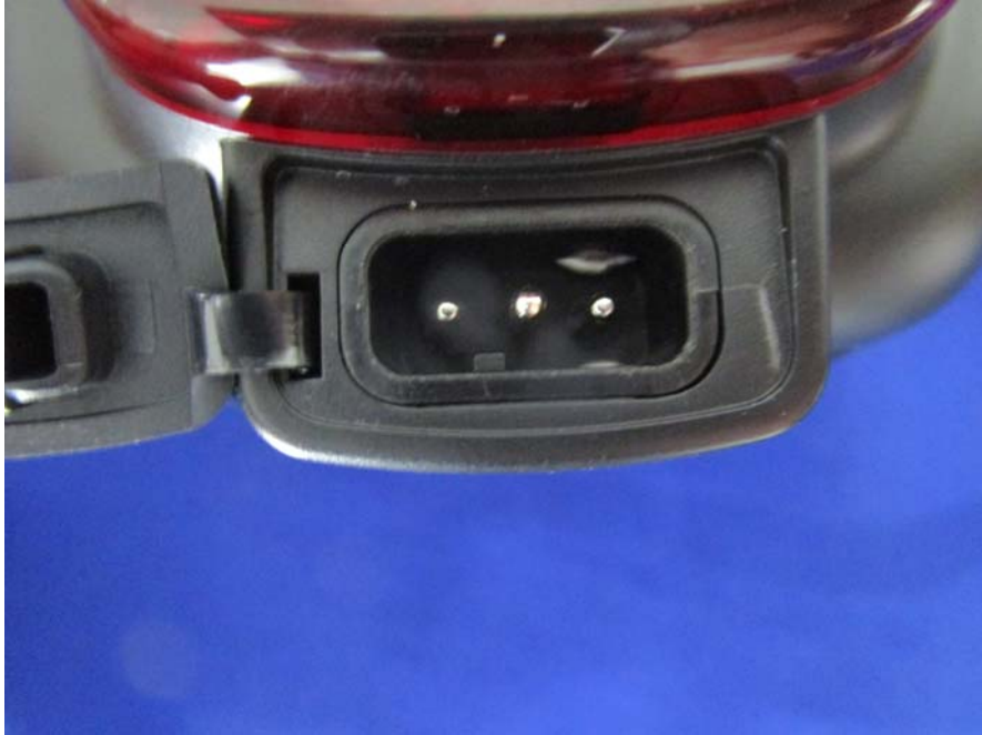
EUT – External Battery Connector View
