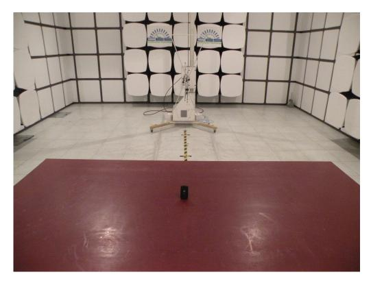
Radiated Emission Test Setup in Chamber
