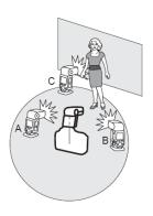
Wireless shooting using radio transmission has advantages over wireless shooting using optic transmission, such as being less affected by obstacles, and not having to point the slave unit's wireless sensor toward the master unit. The main functional differences are as follows:
