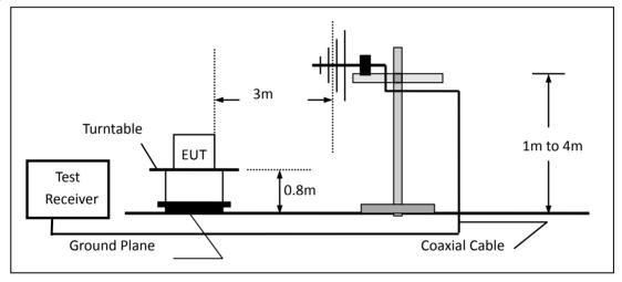
(c) For radiated emissions above 1000MHz
