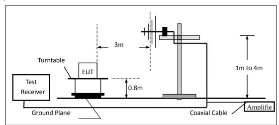
(c) For radiated emissions above 1000MHz
