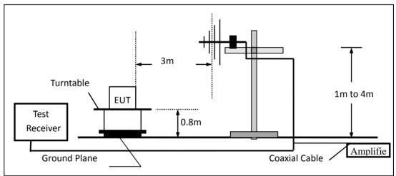
(c) For radiated emissions above 1000MHz
