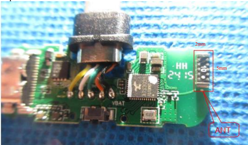
Chip antenna /5.0*2.0*1.0 mm/2400-2500MHz
