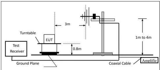
(c) For radiated emissions above 1000MHz
