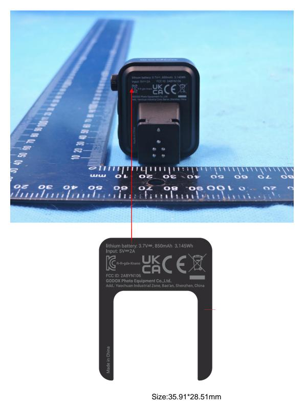
The label is printed on the shielding cover
