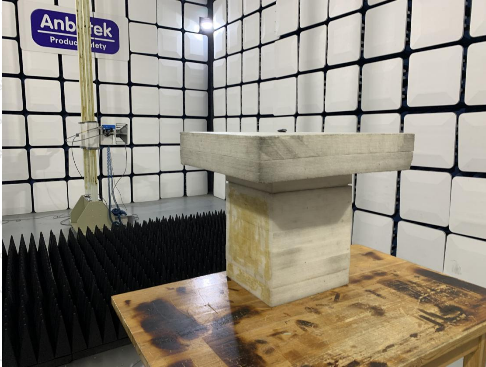
Photo of Radiation Emission Test (above 1GHz)
