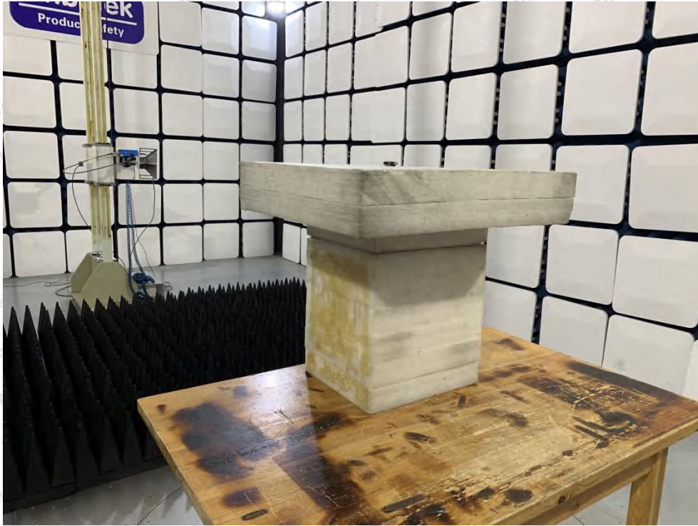
Photo of Radiation Emission Test (above 1GHz)
