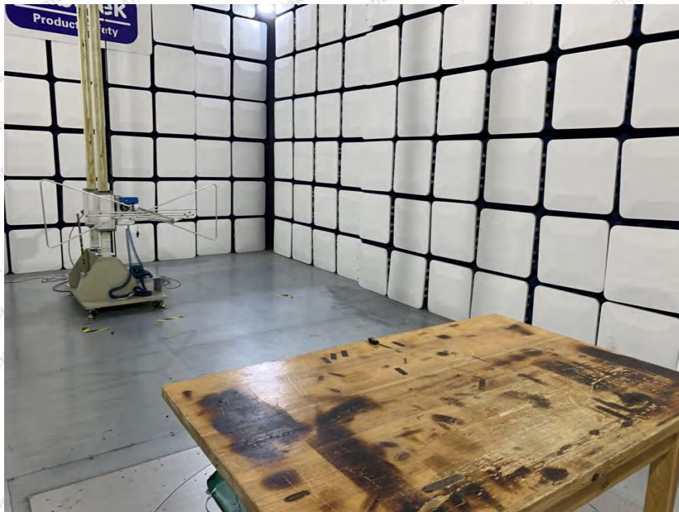
Photo of Radiation Emission Test (below 1GHz)
