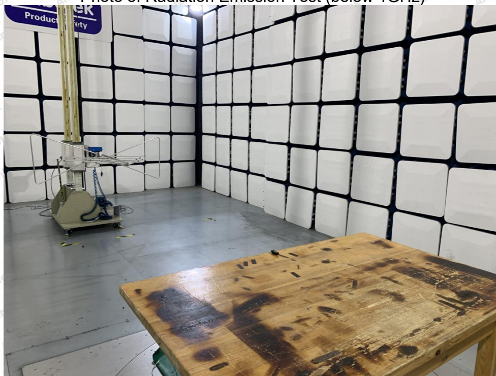
Photo of Radiation Emission Test (below 1GHz)
