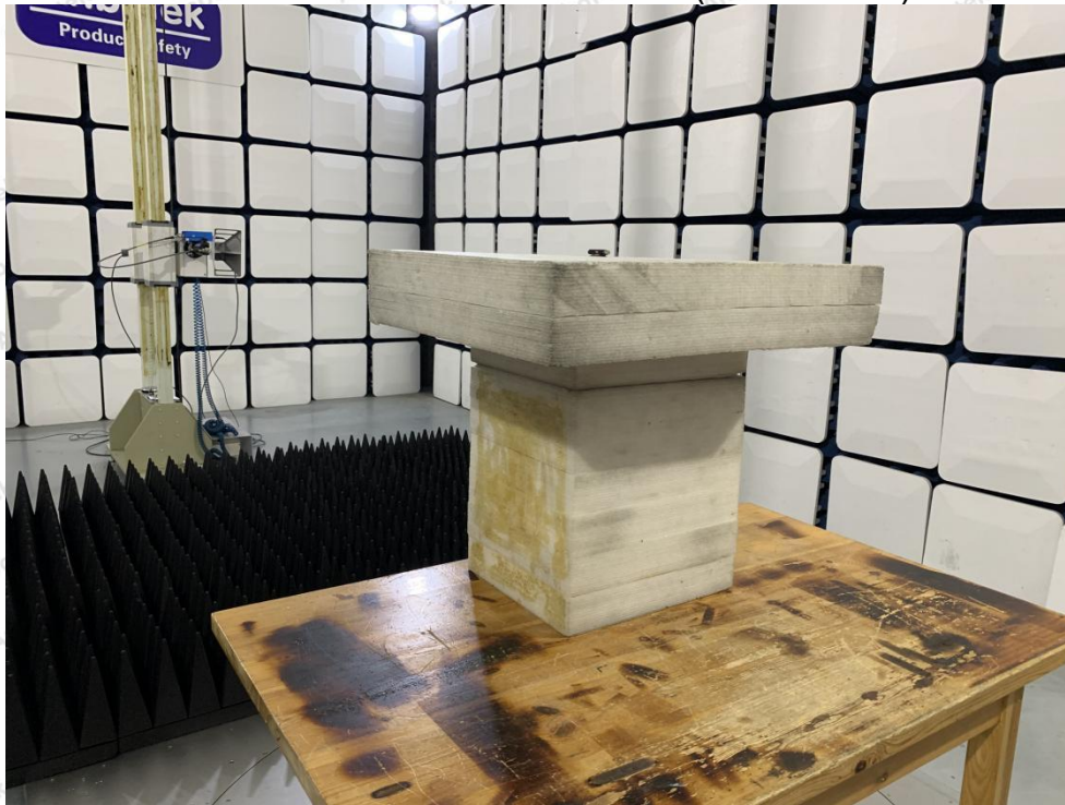
Photo of Radiation Emission Test (above 1GHz)
