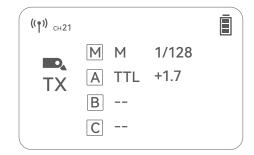
Note: TTL means TTL auto flash, M means manual flash, -- means off.
