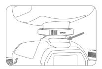
Tightening the lock ring:
