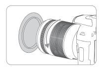
Tips: There are 8 adapter rings applicable to MF-R76C: 49mm, 52mm, 55mm, 58mm, 62mm, 67mm, 72mm and 77mm.
