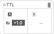
Short press the SET button to select group A flash/group B flash, turn the select dial to adjust the FEB value from -3 to +3 with an increment of 1/3 each stop.
