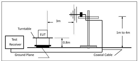
(c) For radiated emissions above 1000MHz
