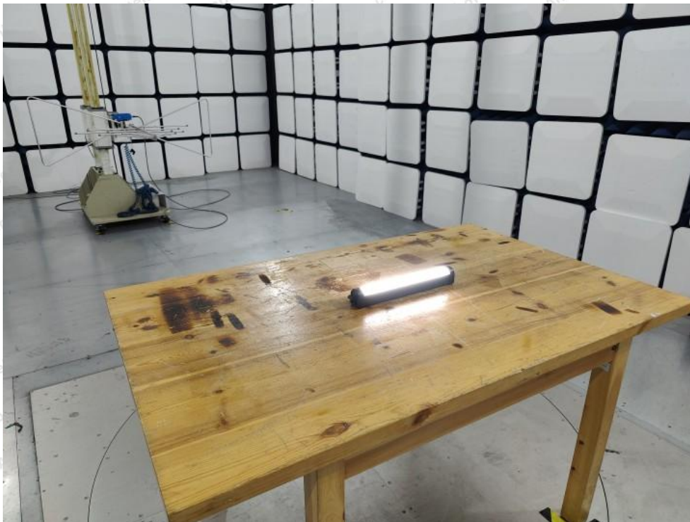
Photo of Radiation Emission Test
