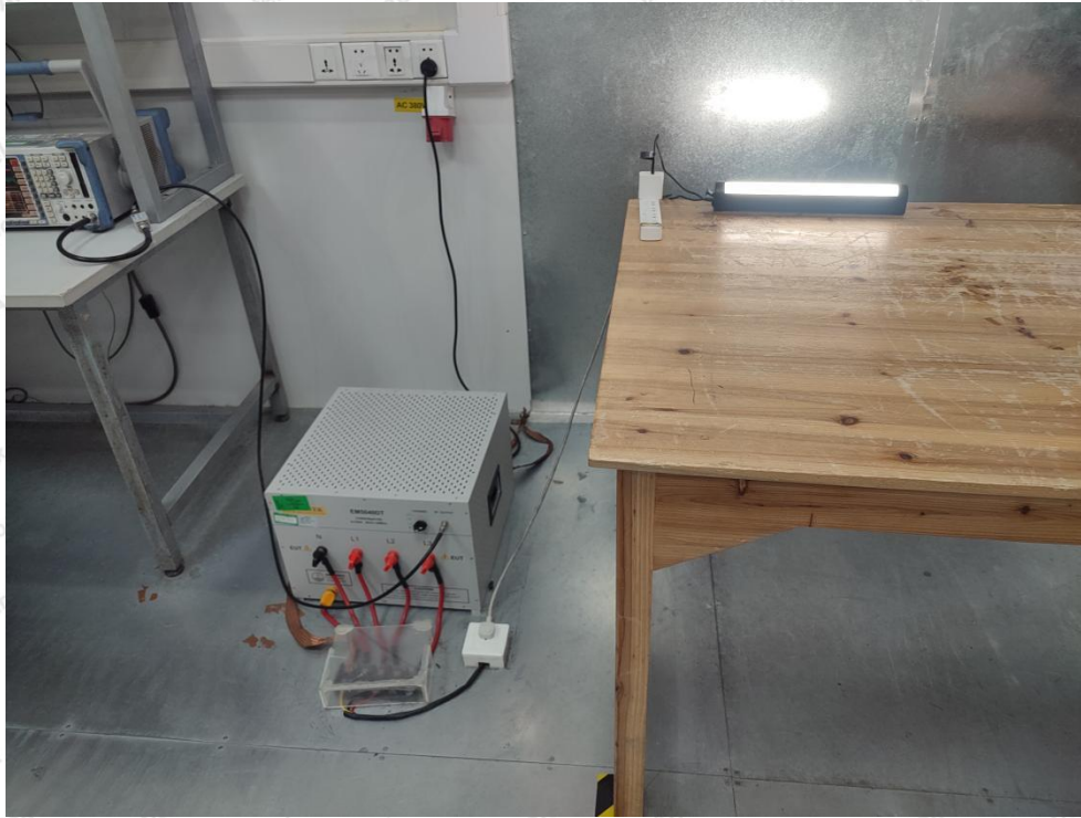
Photo of Radiation Emission Test
