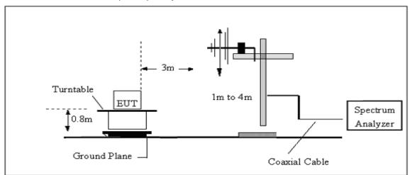
(C) Radiated Emission Test-Up Frequency Above 1GHz
