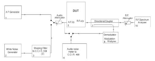
NOTE: If the DUT incorporates ancillary coding or signalling channels, for example, pilot tone, etc. these should be switched on prior to measuring the transmitter RF output spectrum.
