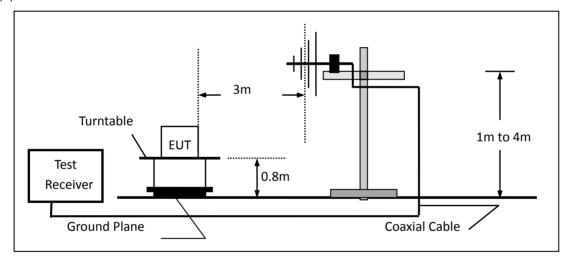
(c) For radiated emissions above 1000MHz
