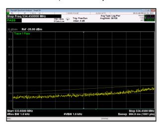
The Average figure with modulation (fc+B ~ fc+1MHz)
