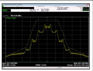
The Average figure with modulation (fc-1MHz~fc-B)
