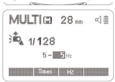
1. Short press the<+/->button to select the flash output value, then rotate the adjustment wheel to adjust the flash output value. After adjustment, short press the setting button to complete the setting.
