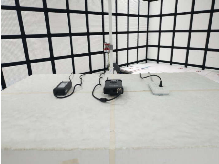
Radiated spurious emission Test Setup-3(Above 1GHz)
