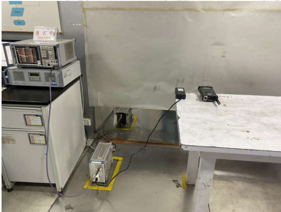
Conducted Emissions Test Setup
