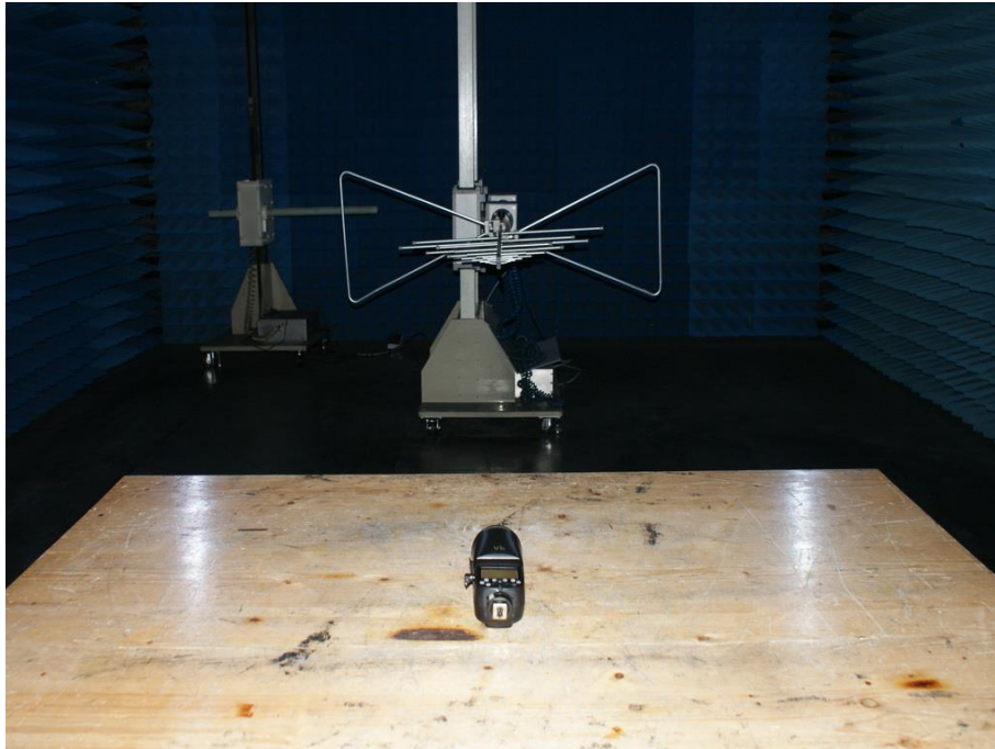
Photograph 3: Set-up for Radiated Spurious Emission, 30MHz - 1GHz
