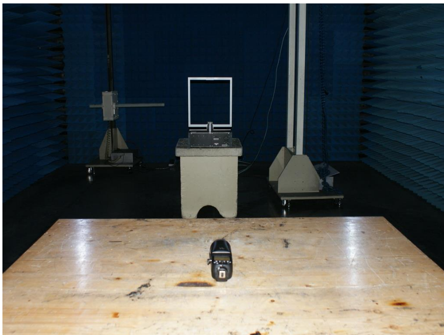
Photograph 2: Set-up for Radiated Spurious Emission, 9KHz - 30MHz
