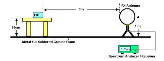
(B) Radiated Emission Test-Up Frequency 30MHz~1GHz
