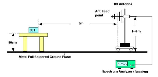
(C) Radiated Emission Test-Up Frequency Above 1GHz
