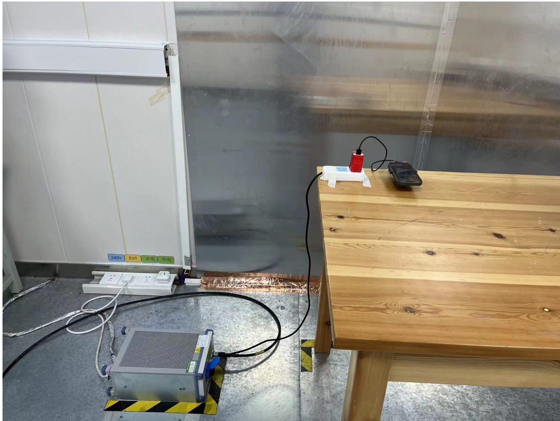
Conducted emission test setup
