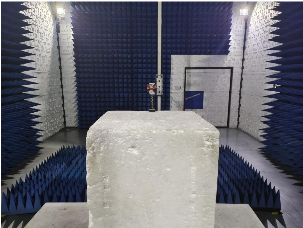
RADIATED EMISSION TEST SETUP ABOVE 1GHz
