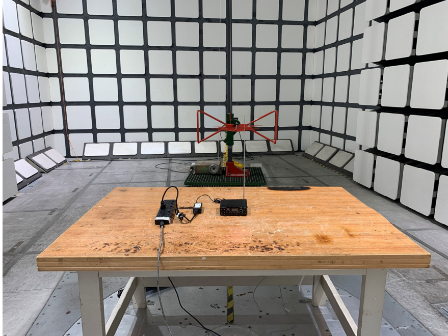
Transmitting Radiated Emissions (Below 1 GHz)
