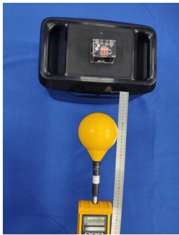
**9.5 Test Position D-Exposure photo from side edge surface-Right**
