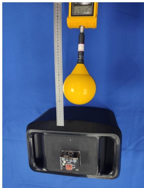
**9.3 Test Position B-Exposure photo from side edge surface-Left**
