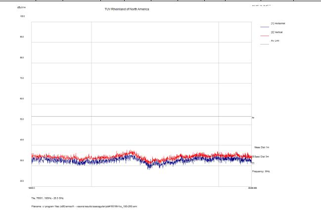
Spec Margin = E-Field AVG - Limit, E-Field AVG = FIM AVG+ Total CF ± Uncertainty Total CF= AF+ Cable Loss AF= Antenna factor + Preamp
