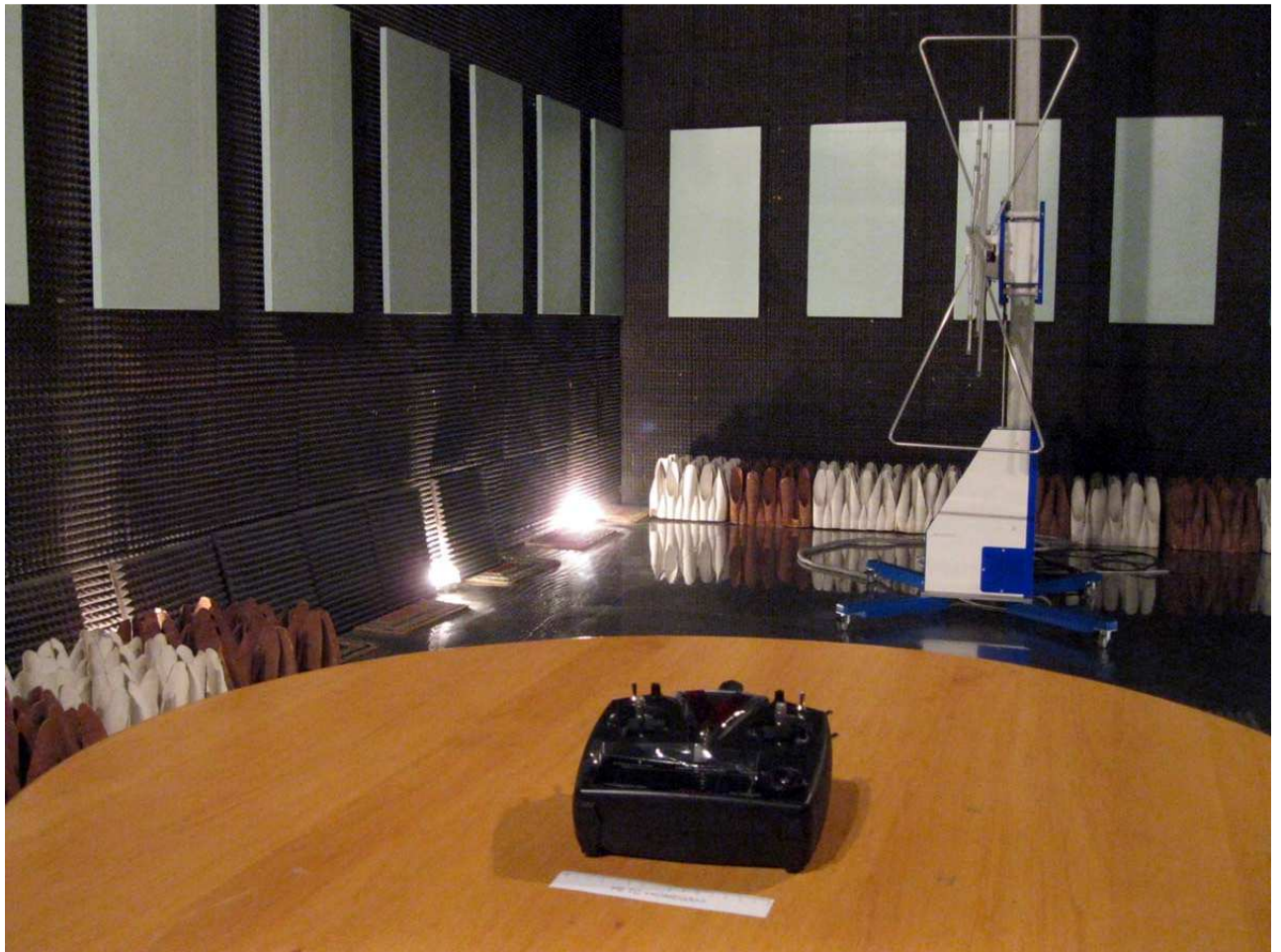
Figure 2.6.2 - Radiated Emission Test (Frequency Range 30 MHz – 1000 MHz)
