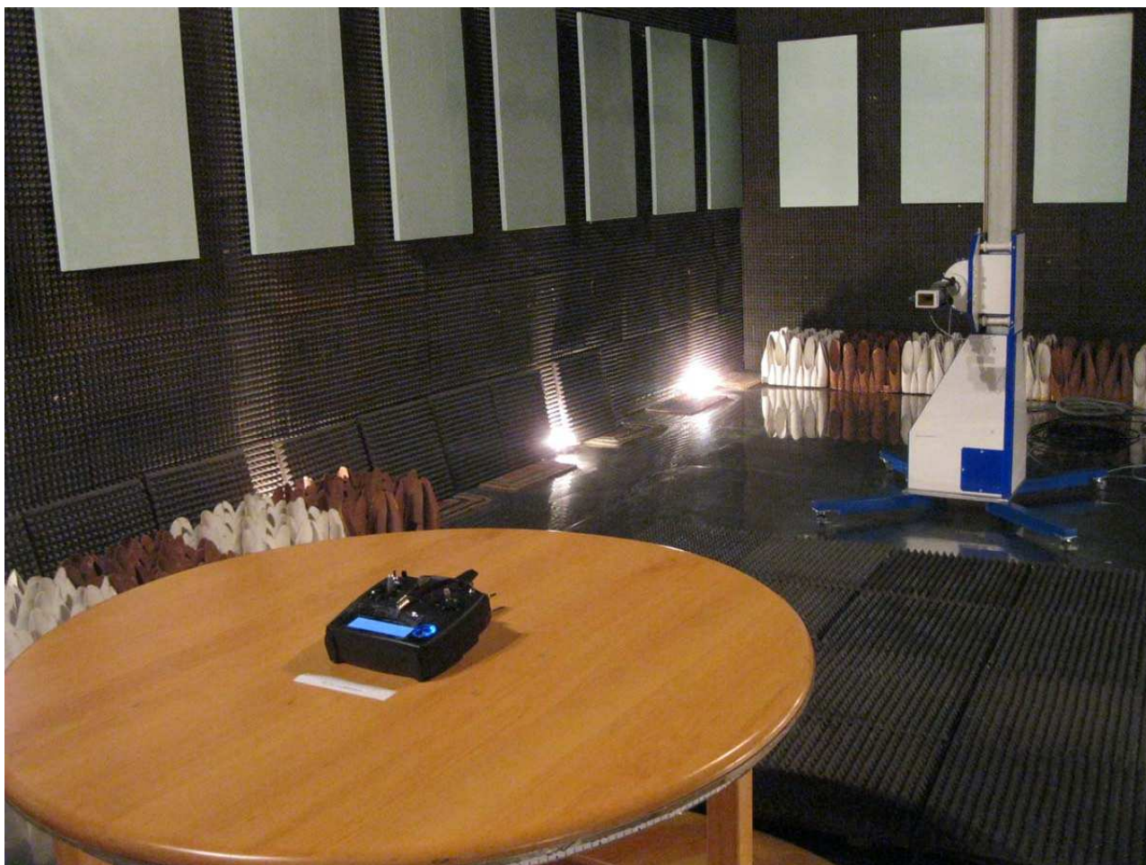
Figure 2.6.4 - Radiated Emission Test (Frequency Range 18 GHz – 25 GHz)
