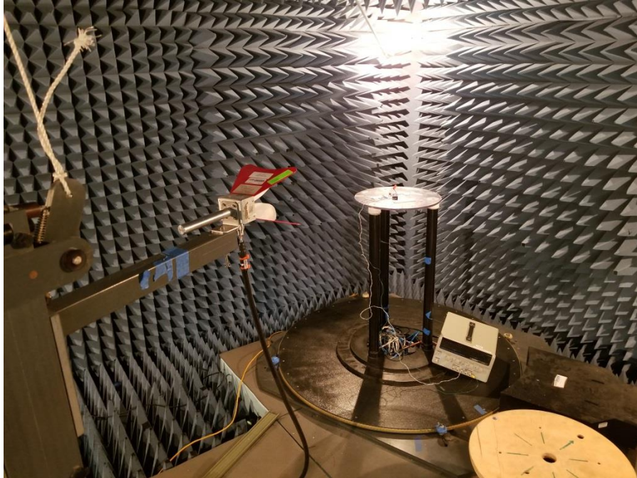
Photograph 1. Radiated Spurious Emissions, Above 1 GHz, Test Setup
