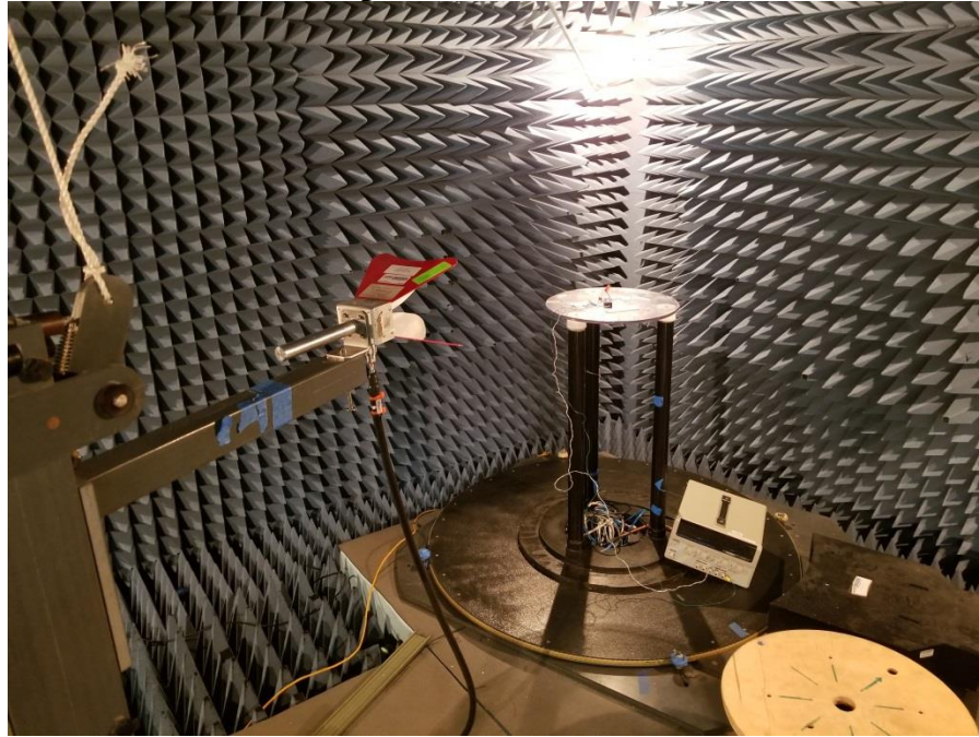
Photograph 1. Radiated Spurious Emissions, Above 1 GHz, Test Setup
