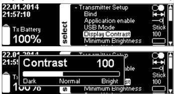
**Minimum Brightness** sets the low threshold of the ambient light sensor. The display will not go darker than the value set here. To save battery life, use the lowest convenient value.
