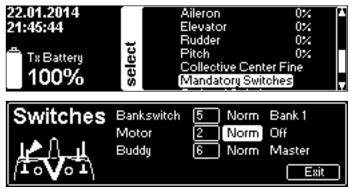
**Optional switches** assigns Option 1-3 functions to switches according to your liking. You will then assign Option functions within additional apps. May require additional hardware and/or software.
