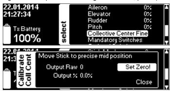
**Mandatory switches** assigns three switches needed for basic flight operations and the directions according to your liking. Defaults are Motor–upper left, Bank switch (flight modes)–upper right, Buddy Box–lower right. The graphics show the actual assignment.
