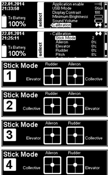
You can calibrate the gimbals by selecting one control function at a time and 'show' the VBar Control the limits and the center position just by moving the stick. It will learn and store the values automatically.
