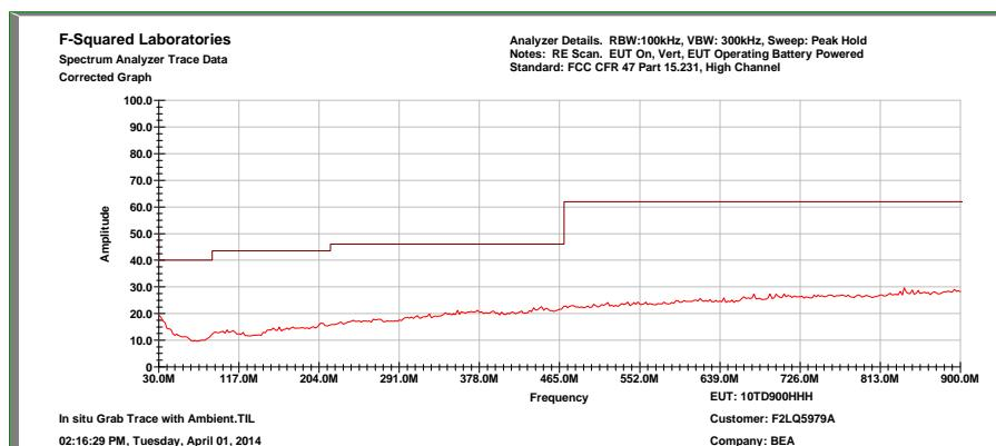
**High Channel: 880 MHz to 1 GHz, Horizontal**
