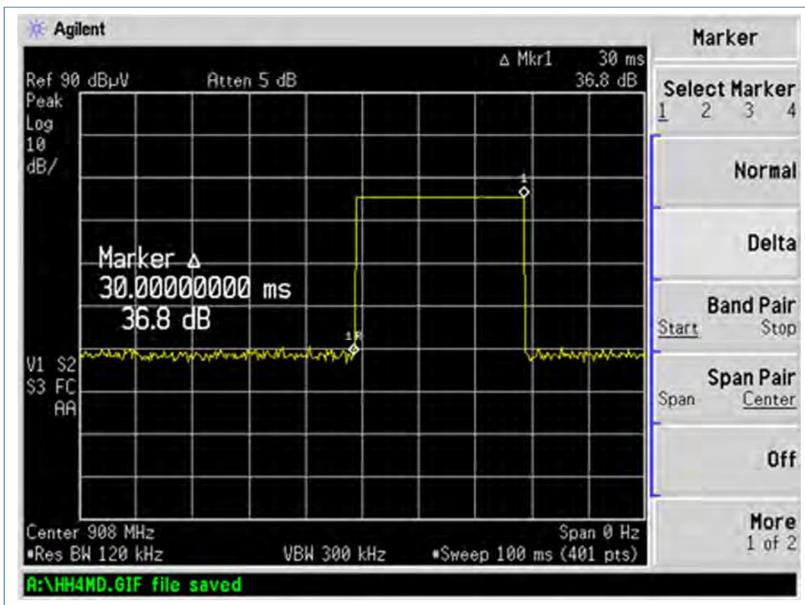
**10 PHOTOGRAHPS****Radiated Spurious Emissions**
