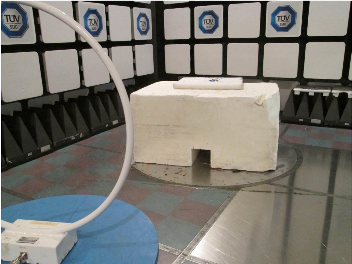
Test setup photo 1 Radiated measurements, 9 kHz – 30 MHz
