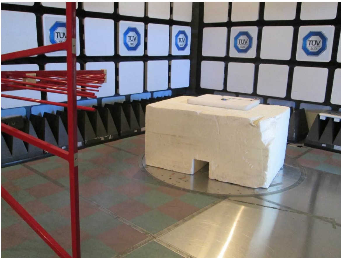
Test setup photo 2 Radiated measurements, 30 MHz – 1 GHz
