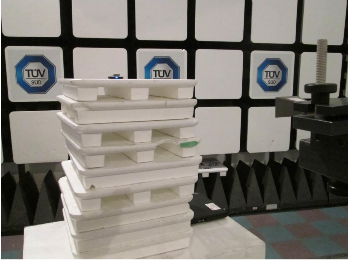
Test setup photo 6 Radiated measurements, 18 GHz – 26 GHz
