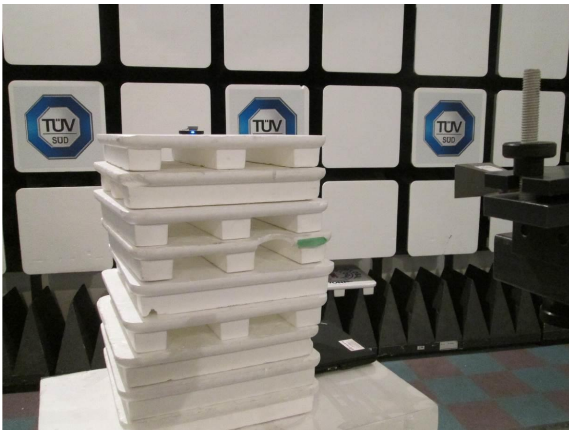
Test setup photo 6 Radiated measurements, 18 GHz – 26 GHz
