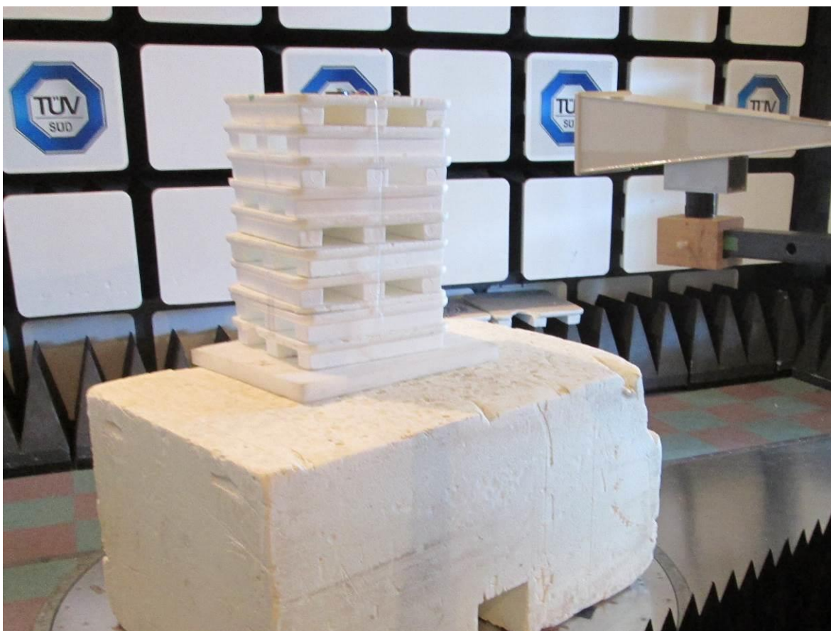
Test setup photo 5 Radiated measurements, 10 GHz – 18 GHz
