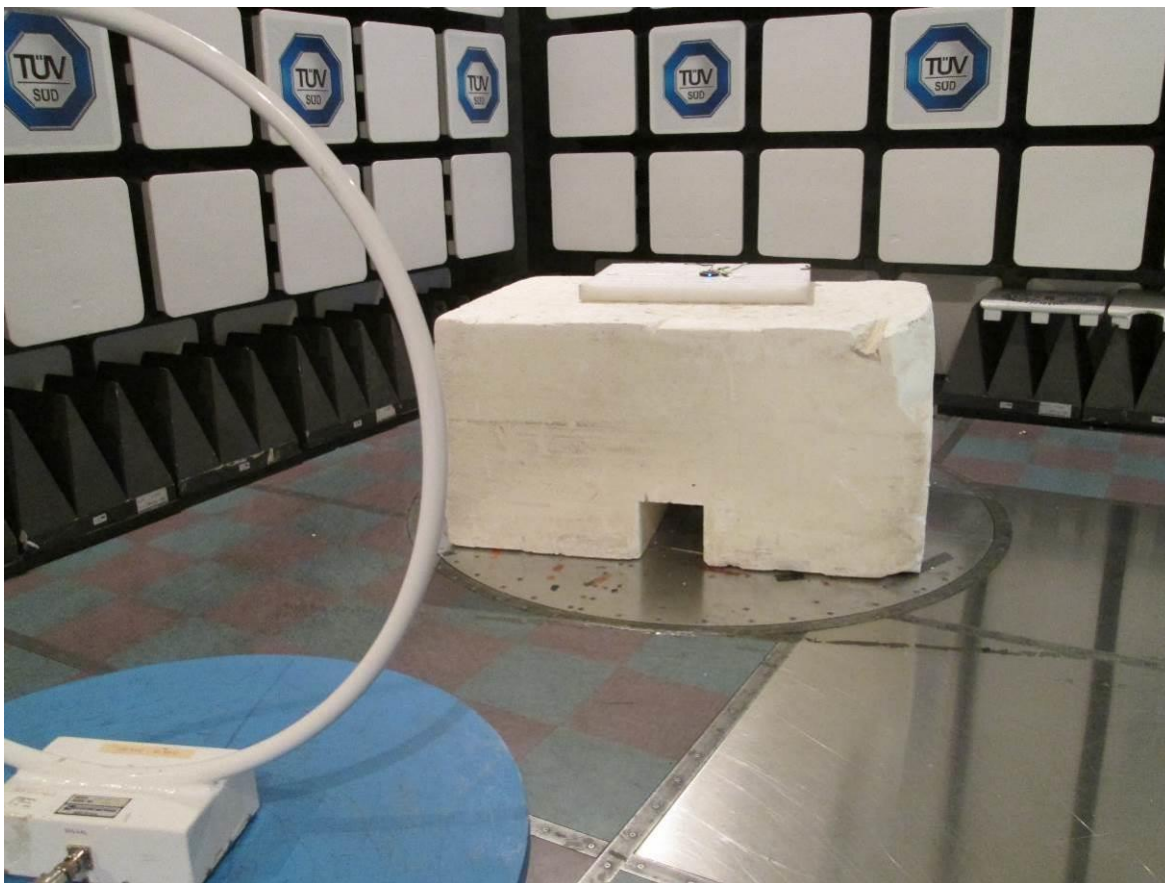
Test setup photo 1 Radiated measurements, 9 kHz – 30 MHz
