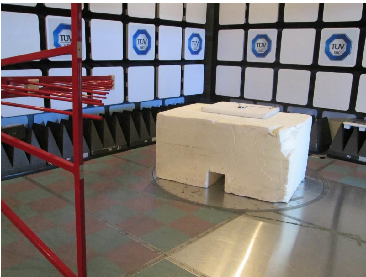
Test setup photo 2 Radiated measurements, 30 MHz – 1 GHz
