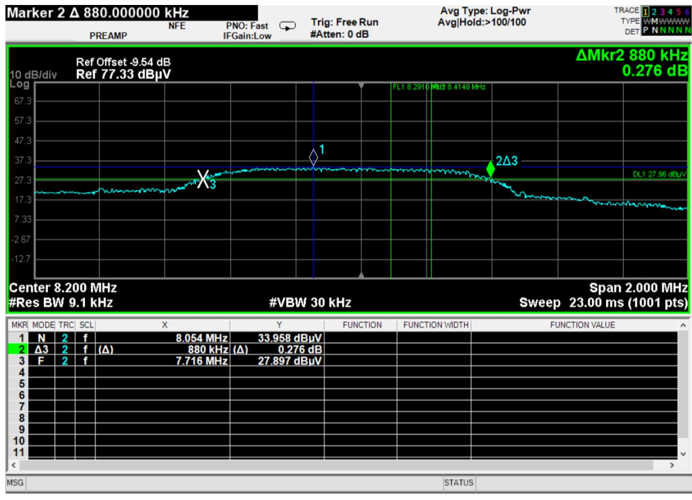
Bandwidth plot to prove emission is at least 10% of the center frequency – 25 Watt Power Supply
