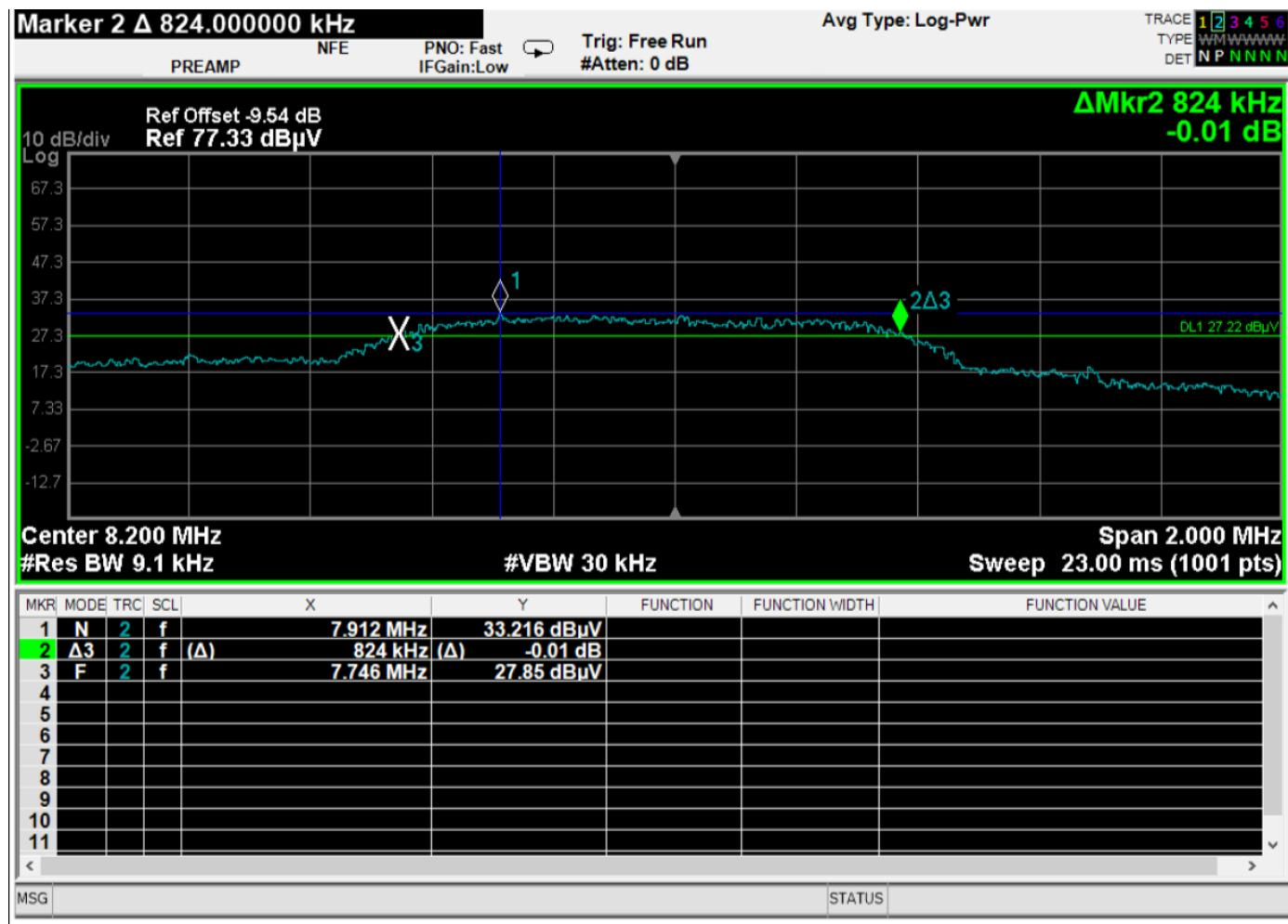
Bandwidth plot to prove emission is at least 10% of the center frequency – 65 Watt Power Supply
