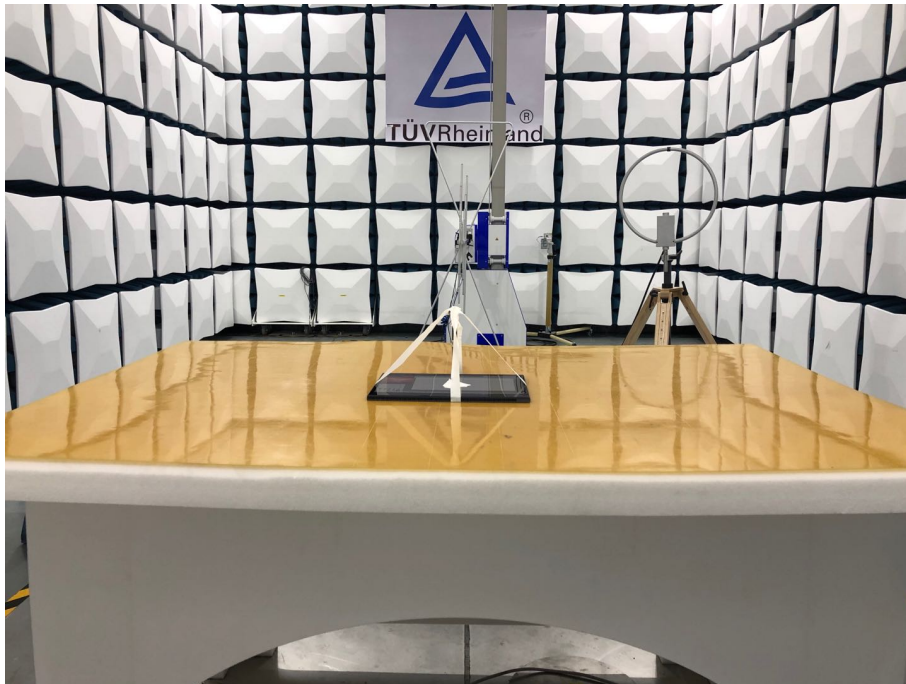
Photograph 6: Set-up for Radiated Spurious Emission, above 1GHz
