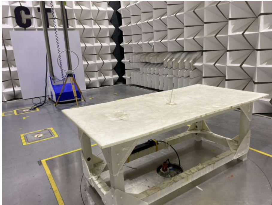
Radiated spurious emission Test Setup-1(Below 30M)
