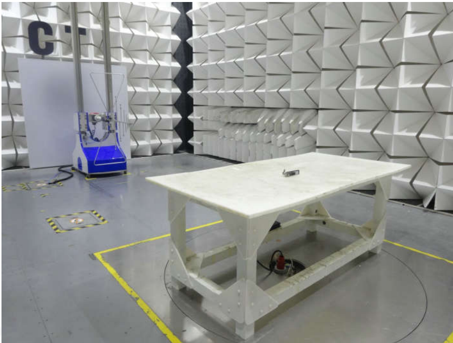
Radiated emission Test Setup (30MHz-1GHz)
