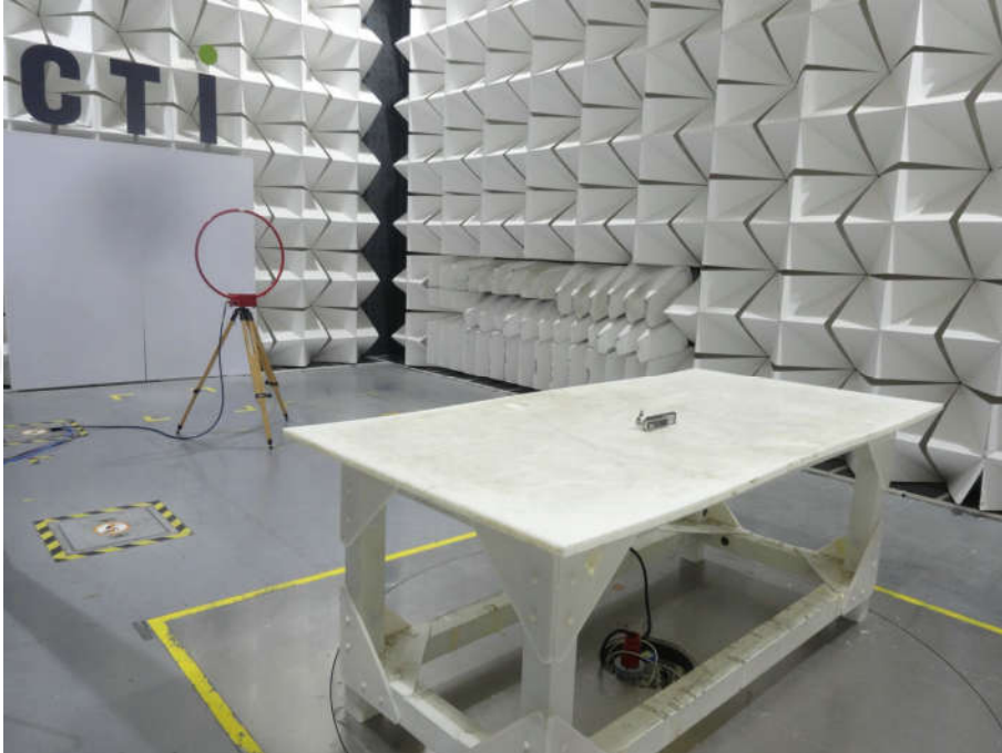
Radiated emission Test Setup (9kHz~30MHz)
