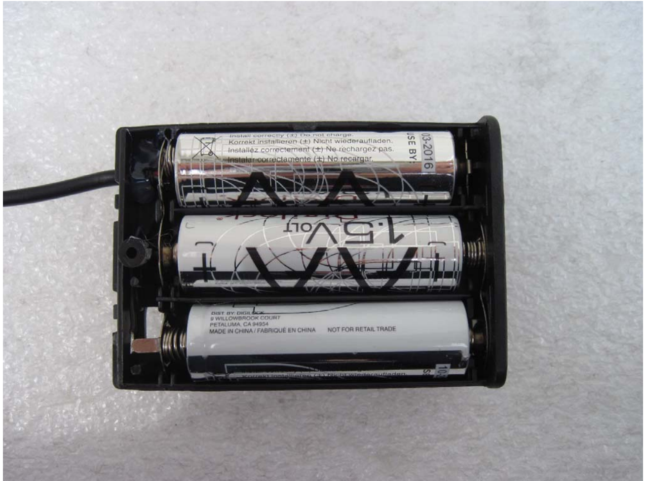
BATTERY PACK INTERNAL VIEW
