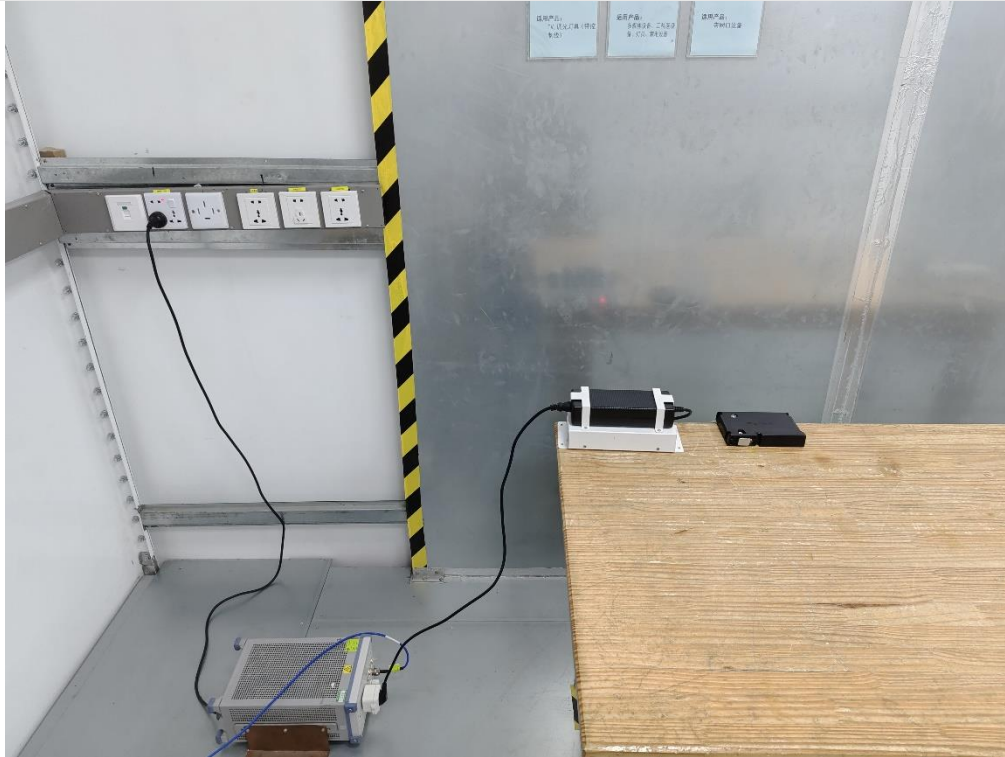
AC Power Line Conducted Emission
