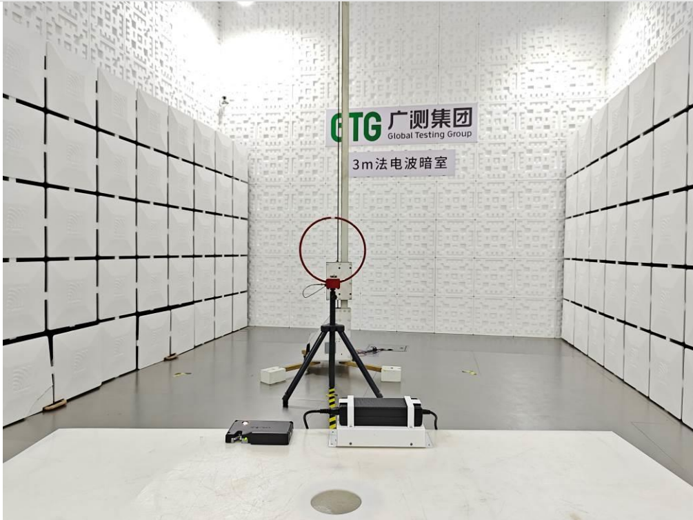
Radiated emissions 9K-30MHz
