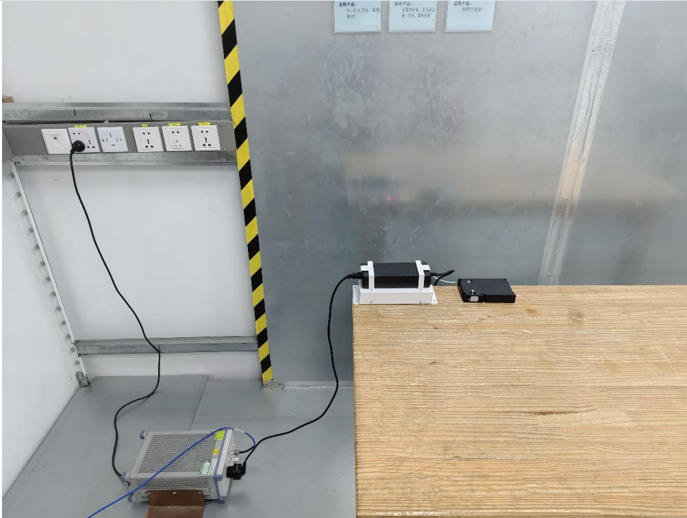
AC Power Line Conducted Emission
