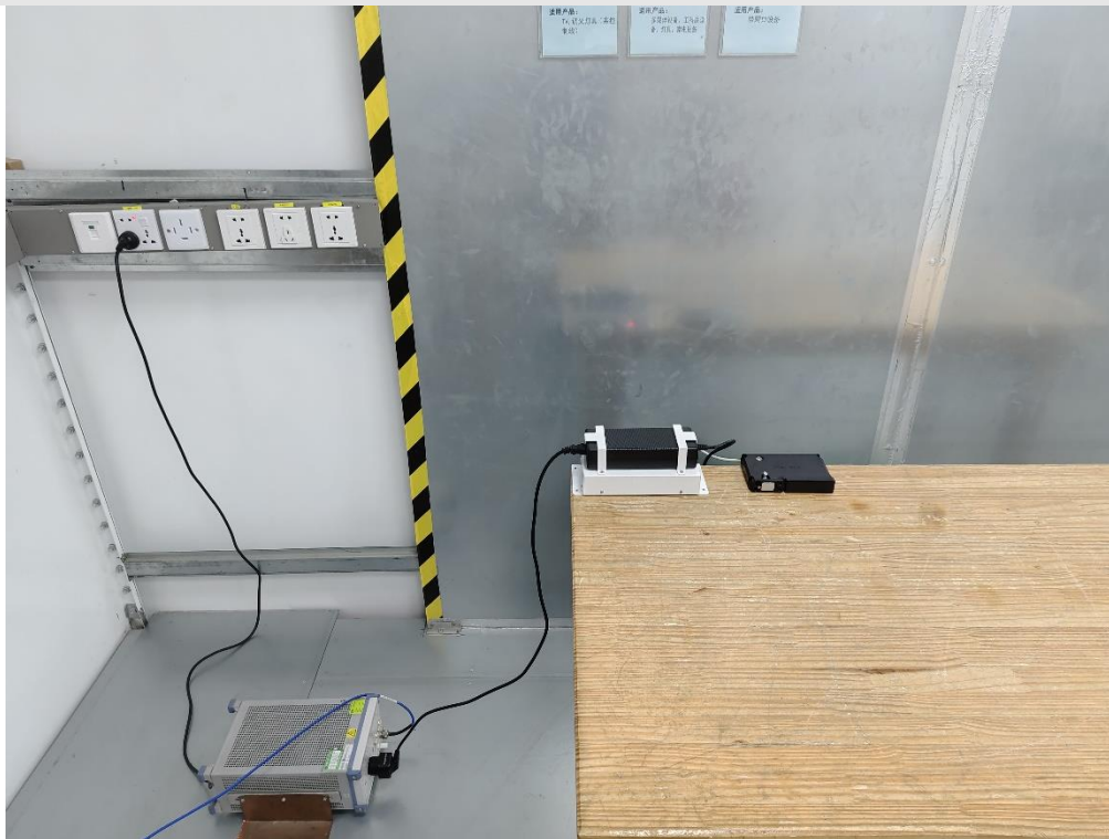
AC Power Line Conducted Emission
