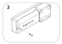
Replace the Cover Plate and secure with the screw.
