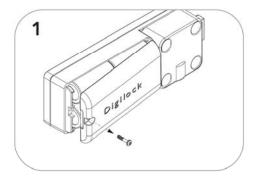
Remove the screw from the Cover Plate with a Phillips head screwdriver.
