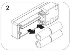
Remove the batteries from the housing. Replace with four premium lithium 123A batteries. Dispose or recycle used batteries according to local regulations.
