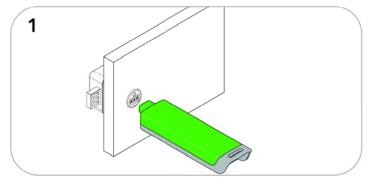
Insert the Power Jumper Key into the key slot. The LED will flash several times, a three tone beep will be heard and the LED will turn off.
