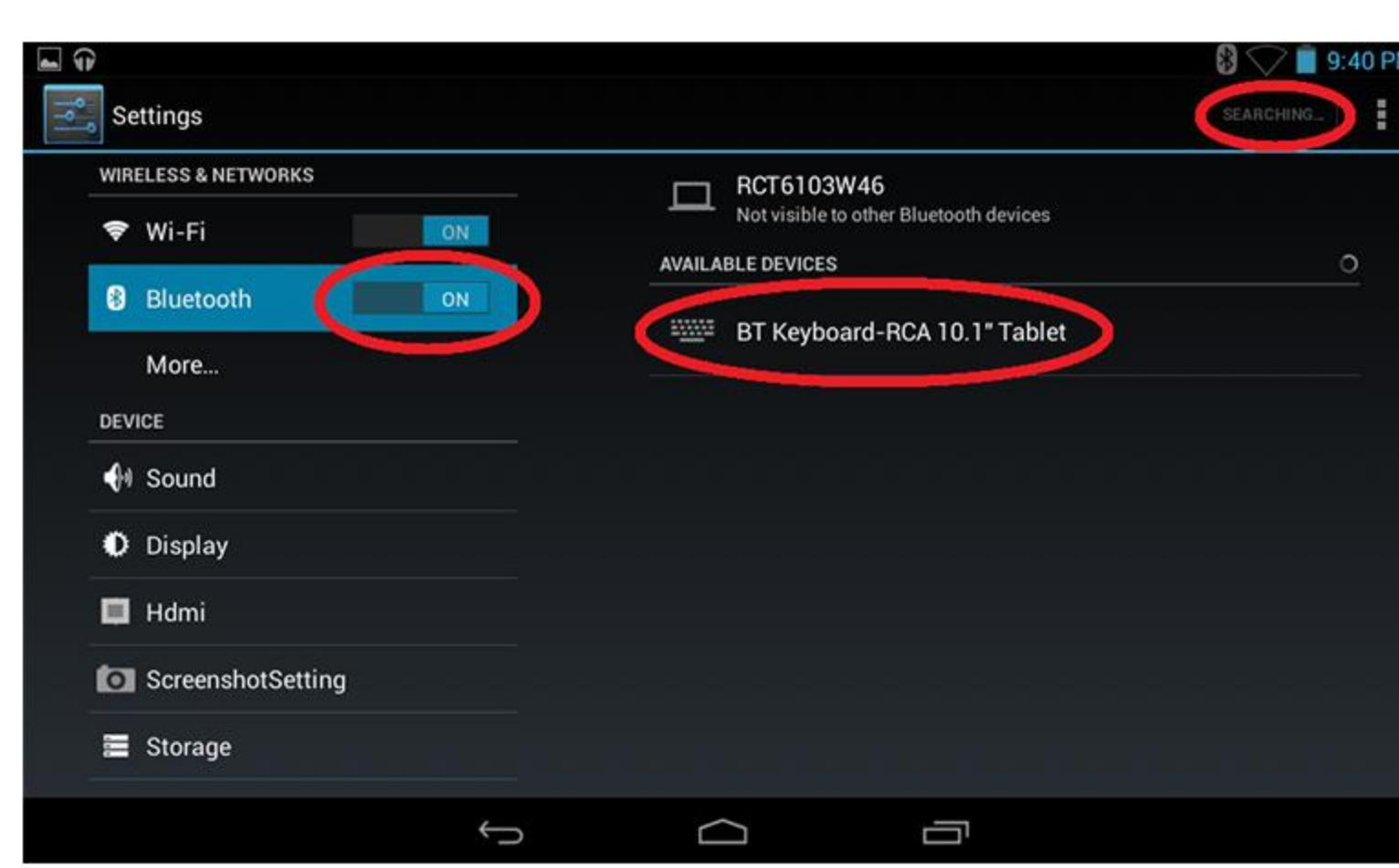
◆ Step3: The implementation of Tap Bluetooth Wireless Keyboard connection. Arabic on-screen prompts for the code, click on the Enter key to connection.
