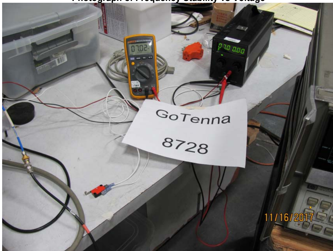
Photograph of Frequency Stability vs Voltage
