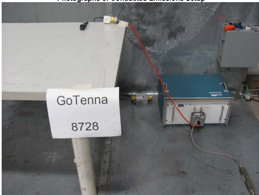
Photographs of Conducted Emissions Setup
