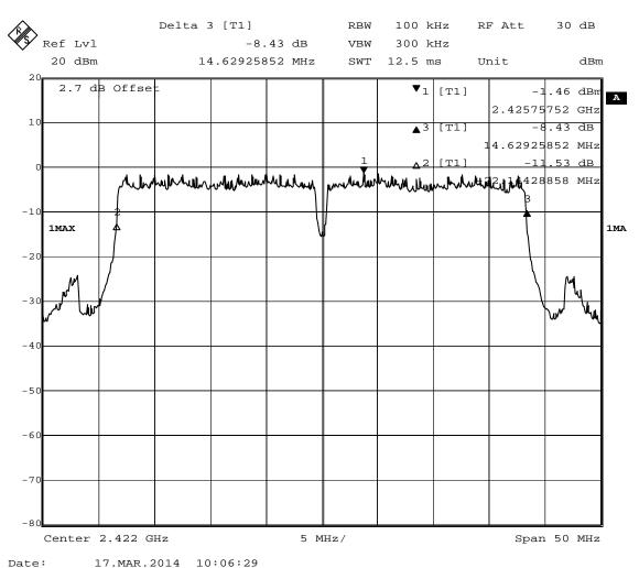
6 dB bandwidth at 2412 MHz, WLAN n-Mode; 40 MHz; 300 Mbit/s
