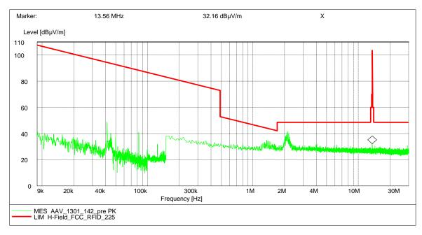
Antenna position 90° EUT position vertical
