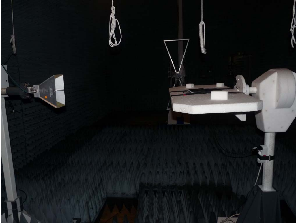
Photo 3: Test setup for radiated measurements (Enclosure, fully-anechoic chamber, 1-18 GHz intentional radiator §15 / 30 MHz – 10/20 GHz §22/24/27)
