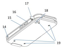
To replace the battery, take of the back cover by loosening all four screws. Take of the back cover. Pull on the battery grip. Pull the battery up.
